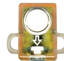
Touch Sensor When is the button touched?
