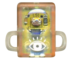
Light Sensor How bright is the light?
